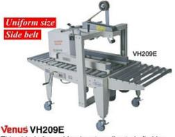
This side belt machine has two direct shaft drive motors: one for each belt. It comes complete with large fore and aft roller bed extensions and lockable castor wheels. Hand adjustable upper guide rollers provide extra carton stability and the taping carriage guide column has a handy carton height scale.
