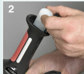
2 Insert the cartridge
