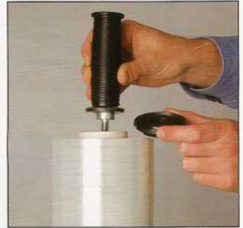
6. Insert the slotted spool end making sure it fits snugly into the roll core. Tighten the handle grip to the desired tension.
