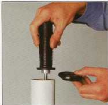
A. Loosen the handle grip enough to remove the slotted spool end, then remove the old film core by sliding it over the handle grip.
