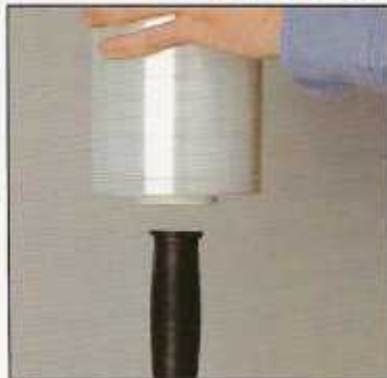
B. Slide the new film roll over the handle grip.
