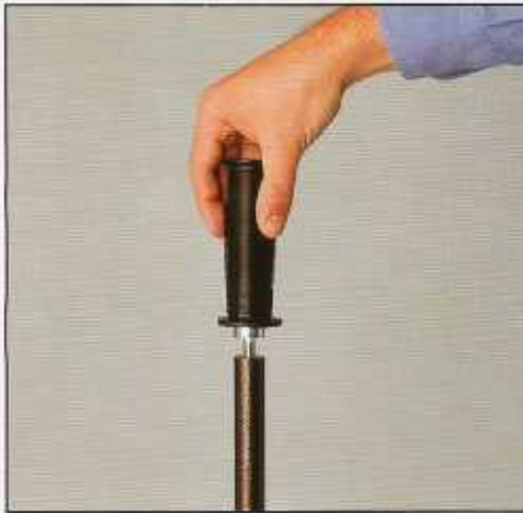
4. Screw the handle grip into the telescopic shaft.
