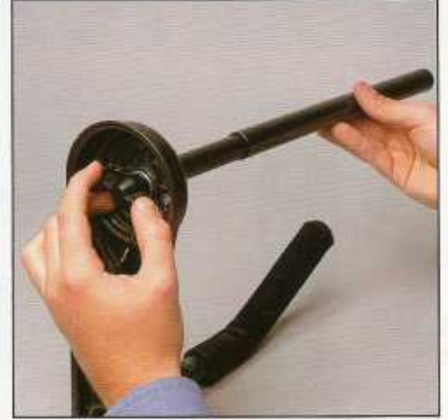
3. Adjust the telescopic shaft to suit the film roll length. Tighten the adjuster wingnut to lock the shaft in position.
