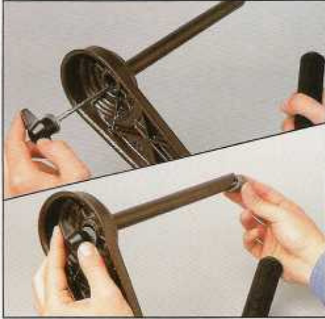
1. Insert the adjuster rod in the bottom shaft. Screw the adjuster rod into the friction lug.
