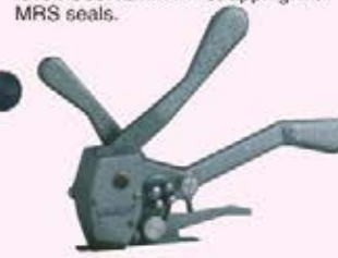
No 78 PP BUNDLER Crimper/tensioner combination. The easy and effective way to bundle pipes, garden stakes, timber etc. Simply insert the seal, lace the strap though it, tension as required, then depress the crimping/cutting lever. Use 12mm PP strapping with MRS seals.
