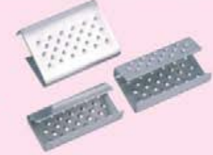
SUPER 4, 5, 6 Indentations penetrate to the inside for a stronger seal. Open flanged, zinc finish. SUPER 4: 12mm wide x 25mm long. Thickness 0.4mm. Available in packs of 2000 and 3000. SUPER 5 and SUPER 6: 15mm wide x 28mm long and 19mm wide x 28mm long. Thickness 0.5mm. 2000 per pack.
